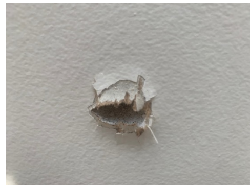
Projectile holes in drywall shot from different angles and different distances.
