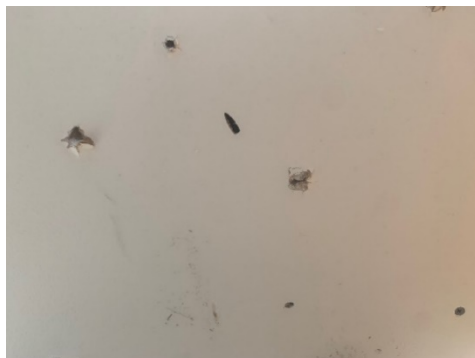
Projectile holes in drywall shot from different angles and different distances.
